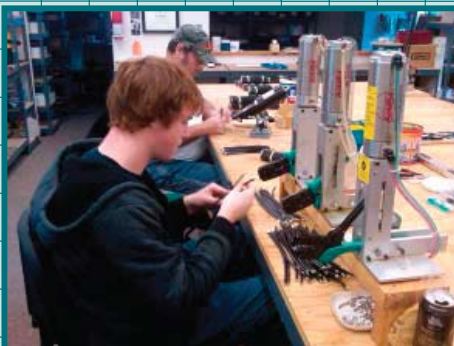
Pneumatic assisted hand tool cylinders insure consistent precise crimps.
